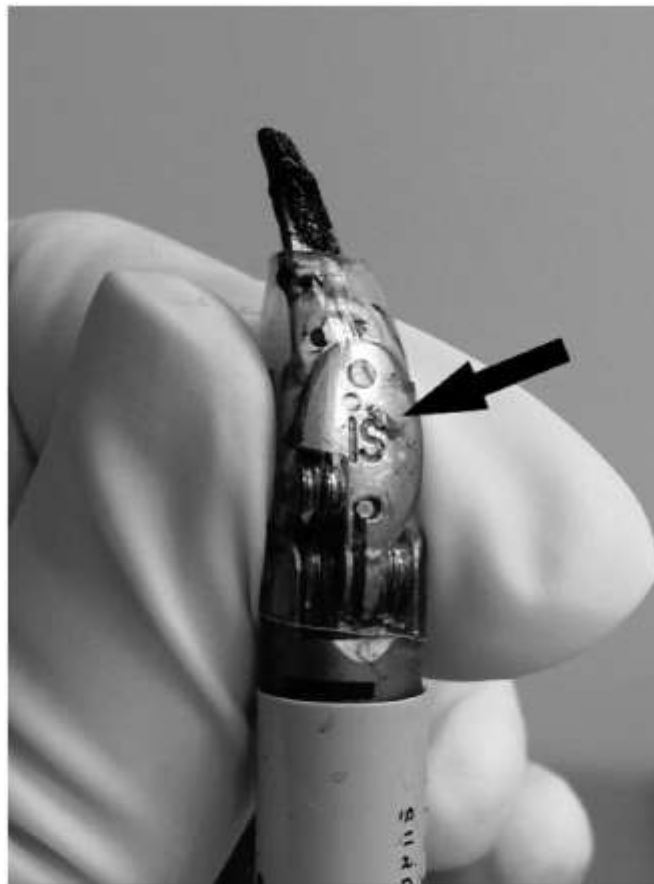
Fig. 1. Cracked plastic sheath after a long surgical case, which led to insulation failure.
